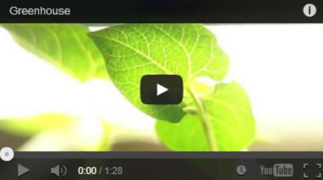
A full-featured, automated greenhouse to grow your indoor plants with peace of mind. Remotely control and monitor light, temperature and humidity. Check the growing process remotely with time-lapse photography. Created with Java Embedded, Raspberry Pi, Pi4J, Arduino, Jetty and multiple sensors.
