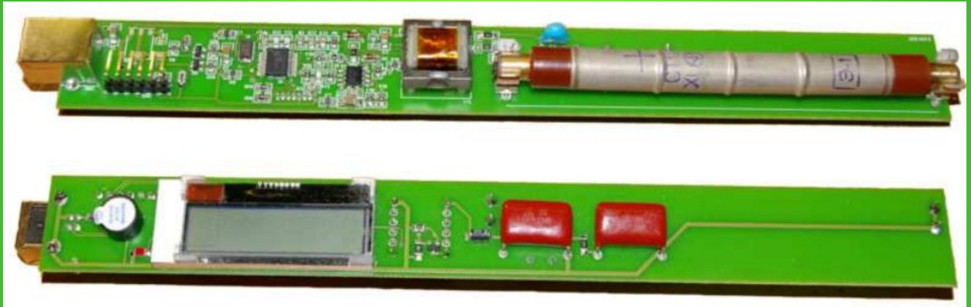
One version of the gamma-ray detector system used in Radioactive@Home
